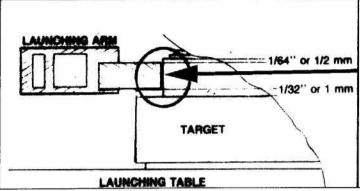
Check the launching arm adjustment with the launcher in the cocked position, viewing the arm and the target from the rear of the machine (refer to illustration at left).
