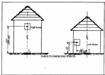
High house; determine the exact position of the targets emerging point in relation to shooting station # 1. The base chord of the field should correspond with the centerline of shooting station 1. The target should be emerging on the centerline of station 1.
